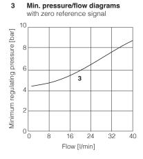
Note: the presence of counter pressure at port T can affect the pressure regulation and the minimum pressure
