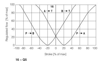
Q5 spool type is specific for alternate P/Q controls in combination with S\* option of digital integral drivers (see tech table **FX500**). It allows to control the pressure in A port or B port and it provides a safety central position (A-T/B-T) to depressurize the actuator chambers.
