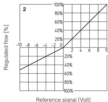
T5 and T7 spool types are specific for fine low flow control in the range from 0 to 60% (T5) and 0 to 40% (T3 and T7) of max spool stroke.
