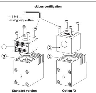
① cover with threaded connection for vertical cable gland fitting (2) cover with threaded connection for horizontal cable gland fitting (3) terminal board for cables wiring
