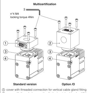
2 cover with threaded connection for horizontal cable gland fitting ③ terminal board for cables wiring
