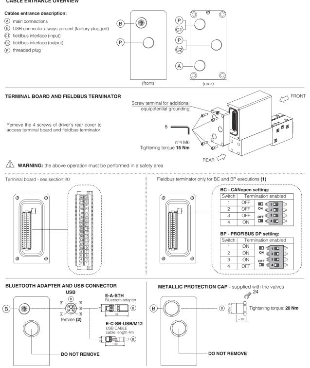
(1) Drivers with BC and BP fieldbus interface are delivered by default 'Not Terminated'. All switches are set OFF (2) Pin layout always referred to driver's view
