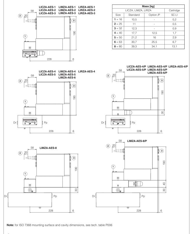
(1) = Screw for air bleeding: at the first valve commissioning the air eventually trapped inside the solenoid must be bled-off though the screw
