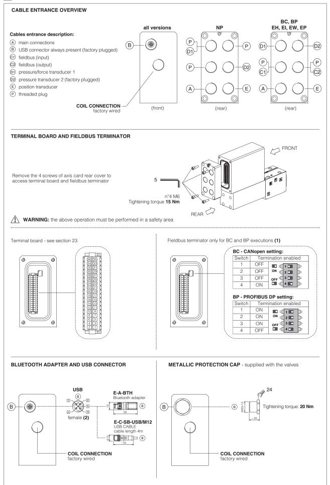
(1) On-board digital driver + axis card with BC and BP fieldbus interface are delivered by default 'Not Terminated'. All switches are set OFF (2) Pin layout always referred to on-board digital driver + axis card view
