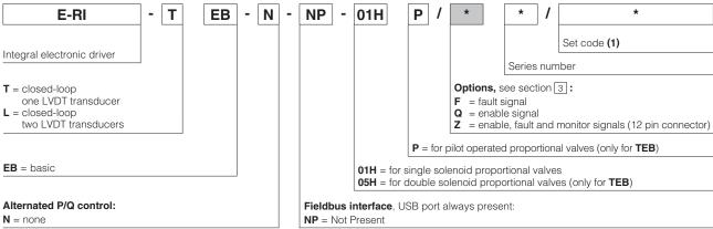
(1) set code identifies the corrispondence between the integral driver and the relevant valve; it is assigned by Atos when the driver is ordered as spare part
