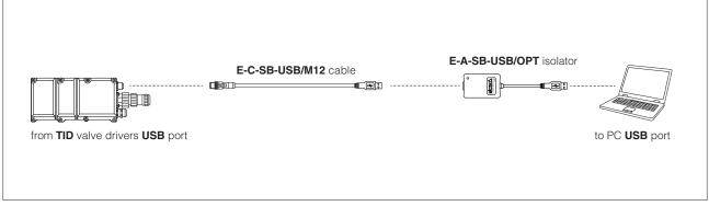
WARNING: the USB port of valve drivers is not isolated and use of USB isolator adapter is highly recommended!
