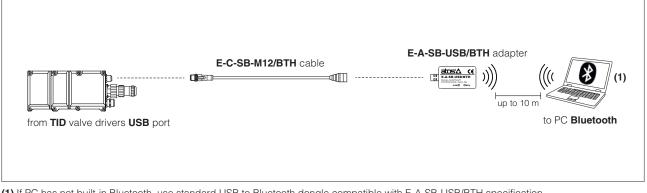
(1) If PC has not built-in Bluetooth, use standard USB to Bluetooth dongle compatible with E-A-SB-USB/BTH specification (please refer to STARTUP-BLUETOOTH guide)
