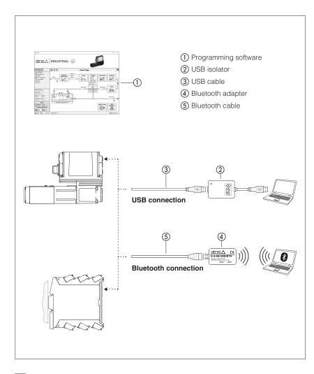
The E-SW and Z-SW programming software are supplied in USB memory stick format and can be easily installed on a desktop or a notebook computer.
