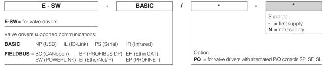
**Notes:** E-SW-FIELDBUS supports also valve drivers without fieldbus communication; E-SW-\*/PQ supports also valve drivers without P/Q control
