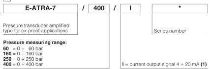
Ex-proof E-ATRA-7 are pressure transducers used to measure the static and dynamic pressure.
