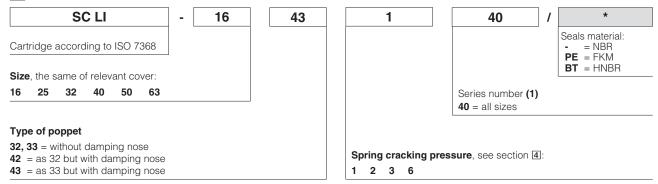
(1) New series 40 is mechanically interchangeable with standard flow series 31, 11 and 10 - cavity according to ISO 7368 New series 50 of LIDD cover is highly recommended in combination with new cartridges series 40 The use of old cartridges series 10, 11 and 31 may cause the impossibility to fully close the poppet
