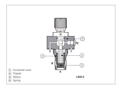
LIDD are flow control valves not compensated, in ISO cartridge design, made by a functional "cover" ① and a 2-way SC LI slip-in cartridge.
