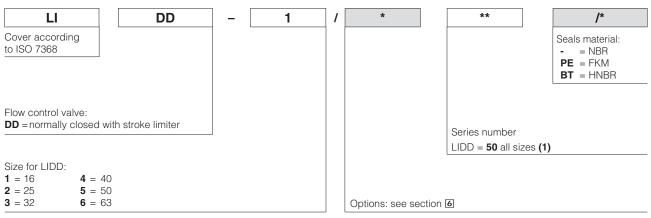
(1): New series 50 of LIDD cover is highly recommended in combination with new high flow cartridges series 40 The use of old cartridges series 10, 11 and 31 may cause the impossibility to fully close the poppet
