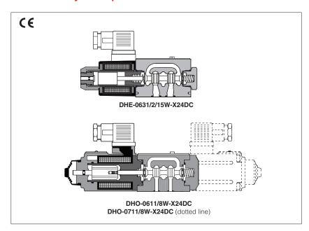
On-off directional valves derived from standard versions and equipped with low power consumption solenoids. They permits a considerable energy saving and they can be directly operated from the output stage of the machine control system (PLC I/O modules)
