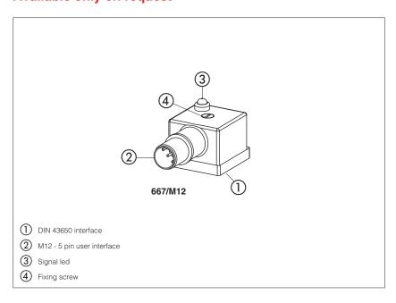
Electric connectors with standard DIN 43650 solenoid interface and M12, 5 pin interface to the user side.
