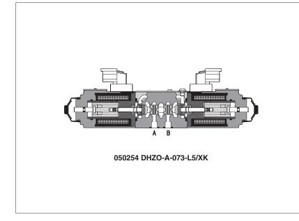
Proportional valves with special Deutsch connector for improved protection to water and atmospheric agents, typical for mobile applications.
