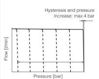
Pump max pressure open loop proportional control.
