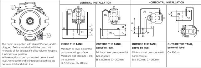
IN: inlet line - D2: drain line - B+C: permissible suction height - C: inlet line immersion dept
