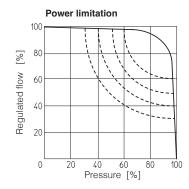
The power limitation algorithm allows to limit the hydraulic power of the pump to the value set via software or fieldbus see section 22.12
