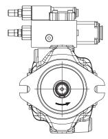
Pumps with counterclockwise rotation (\$) have the IN and OUT inverted and consequently the position of the electrohydraulic proportional controls
