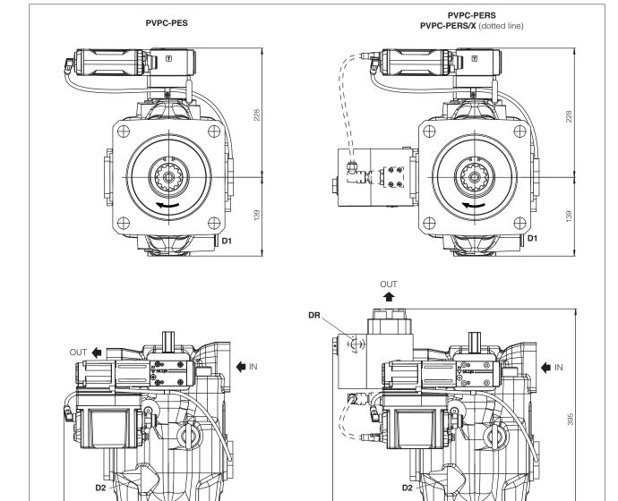
① = Proportional valve with on-board driver with p/Q control
