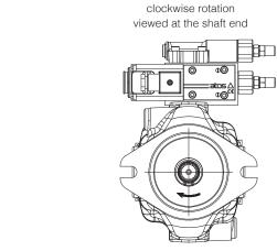
Pumps with clockwise rotation (**D**) have the IN and OUT as shown in all representation of catalogue
