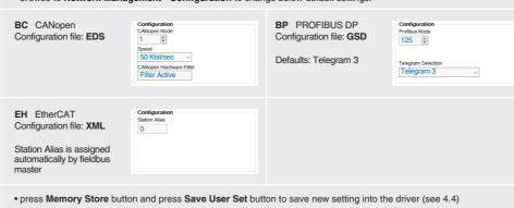
• network configuration settings will be applied at next driver power on or pressing the Restart button
