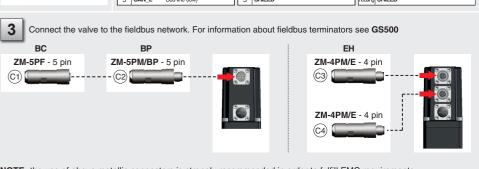
**NOTE:** the use of above metallic connectors is strongly recommended in order to fulfill EMC requirements
