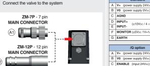
NOTE: the use of above metallic connectors is strongly recommended in order to fulfill EMC requirements
