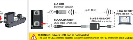
Launch the PC software using E-SW-SETUP icon: 3 PC software does NOT detect valid connection communication is not established, please follow wizard procedure 4 • PC software detects valid connection communication automatically established - valve is **ON-LINE** see 5
