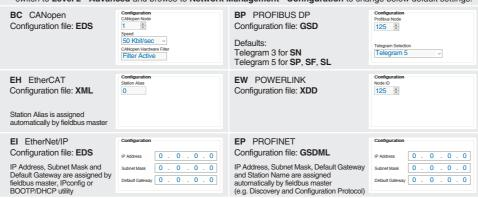
• press Memory Store button and in Fieldbus Parameters press Store User button to save new setting into the driver (see 4.6)
