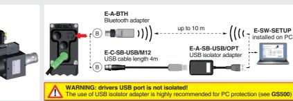
Launch the PC software using E-SW-SETUP icon: 3 • PC software does NOT detect valid connection
