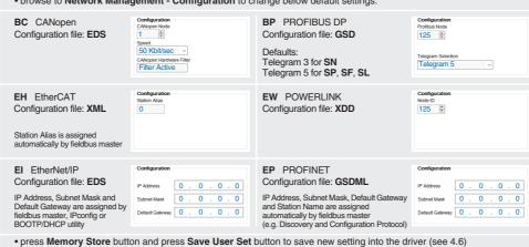
• network configuration settings will be applied at next driver power on or pressing the Restart button
