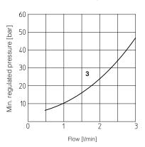
Note: the presence of counter pressure at port T can affect the pressure regulation and the minimum pressure
