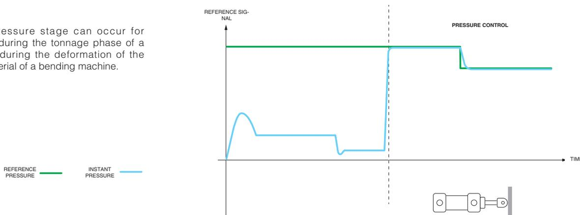
If, during the pressure control phases, a line depressurization is required, the PGI/PGIL pump is able to rotate in the opposite direction for a short period of time.
