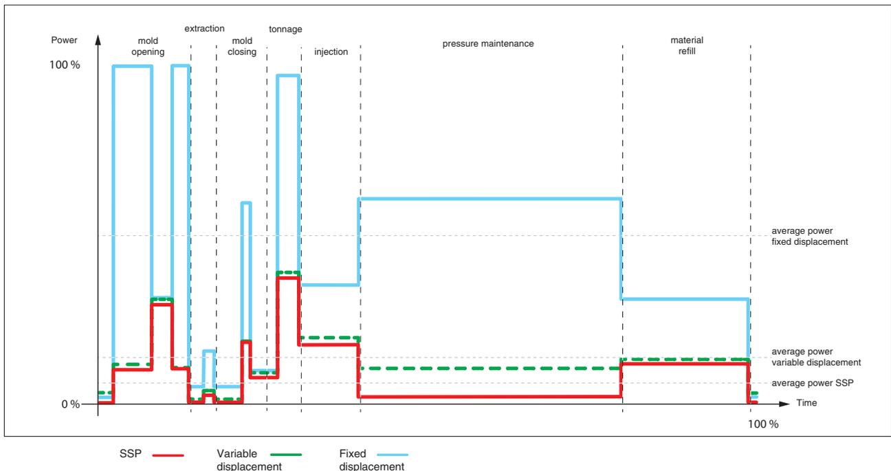
In the graph it is possible to detect in detail the great advantages of SSP in term of energy saving compared to other traditional systems.
