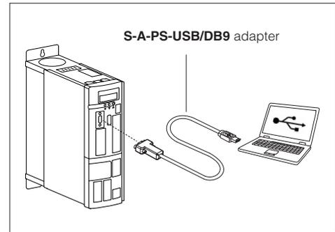
All parameters available on the drive can be monitored with S-SW-SETUP or shared with the customer's PLC via fieldbus
