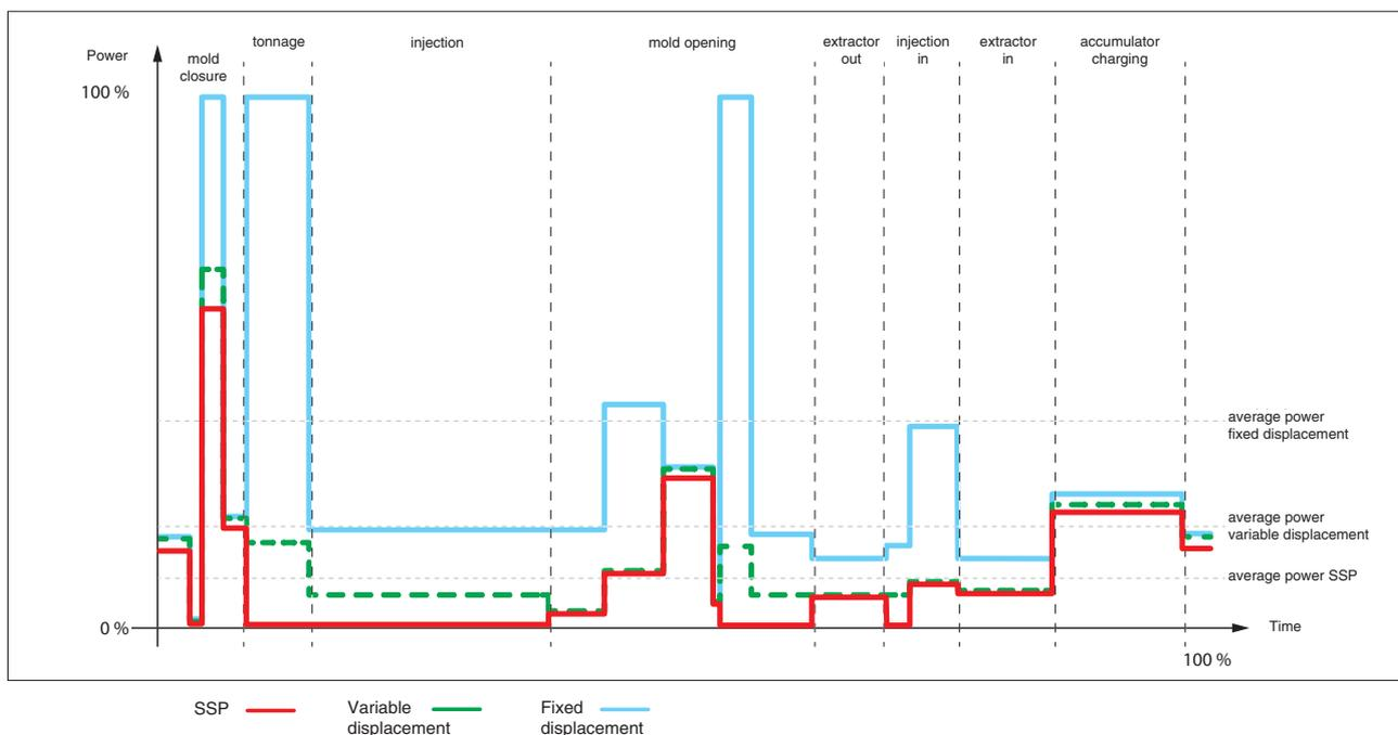
In the cycle shown in the graph, the SSP pump ensures energy savings of up to 65% compared to traditional systems.
