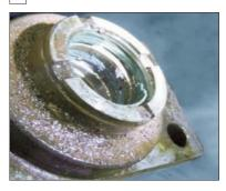
**Trouble description:** very high or low temperatures may cause the seals overheating or freezing, thus the loss of elastic properties and oil leakages. High temperatures make the seals dark and flaked, low temperatures make the seals brittle with heavy damages and may cause breaks in the most stressed and exposed components.
