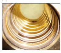
**Trouble description:** cylinders are designed to provide axial force and motion to a guided load, the result of a poor alignment is the excessive side loading of the rod, which involves a premature wear of the bronze bushing, seals and wear rings. Bronze bushing presents a glossy area on one side, seals and guide rings are heavily worn.
