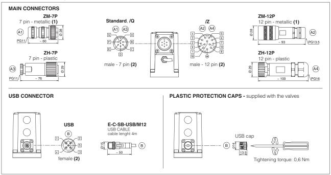
(1) Use of metallic connectors is strongly recommended in order to fulfill EMC requirements (2) Pin layout always referred to driver's view
