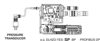
one remote pressure transducer has to be installed on the actuator's port to be controlled. In this example the SP option regulates the pressure on port A
