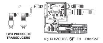
two remote pressure transducers have to be installed on the actuator's ports A and B.
