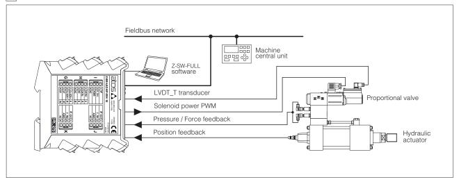
Note: block diagram example for alternated position/force control, with fieldbus interface
