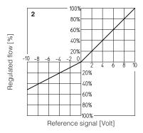
T3, T5 and T7 spool types are specific for fine low flow control in the range from 0 to 60% (T5) and 0 to 40% (T3 and T7) of max spool stroke.
