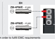
NOTE: the use of above metallic connectors is strongly recommended in order to fulfill EMC requirements
