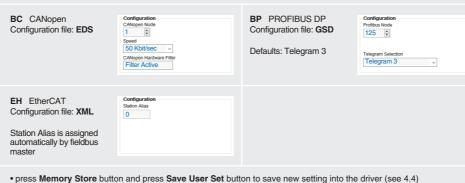
• network configuration settings will be applied at next driver power on or pressing the Restart button
