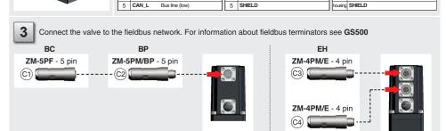
**NOTE:** the use of above metallic connectors is strongly recommended in order to fulfill EMC requirements
