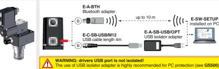
Launch the PC software using E-SW-SETUP icon: • PC software does NOT detect valid connection communication is not established, please follow wizard procedure 4 • PC software detects valid connection communication automatically established - valve is **ON-LINE** see **5**
