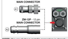
NOTE: the use of above metallic connectors is strongly recommended in order to fulfill EMC requirements
