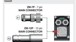
NOTE: the use of above metallic connectors is strongly recommended in order to fulfill EMC requirements
