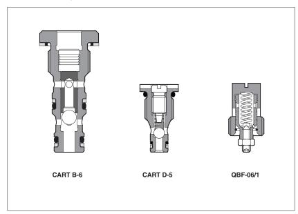
Cartridge valves for piloting lines and load sensing blocks
