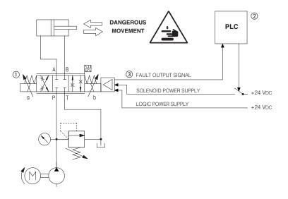
**Safety function** = to prevent the dangerous cylinder movement in a certain phase of the cycle or in emergency
