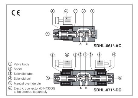
Spool type, two or three position direct operated valves size 06 in compact execution with reduced solenoids dimensions, ideal for applications in mini power packs, mobile and agricultural machines.
