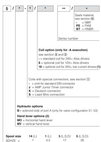
(1) Select coil voltage /18 in case of electronic drivers not supplied by Atos, with power supply 24 VDC
