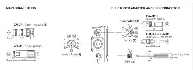
(1) use of metallic connectors is strongly recommended in order to fulfill EMC requirements
