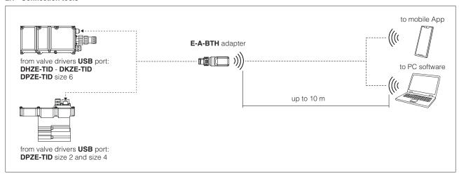
(1) The previous versions of the Bluetooth adapter E-A-SB-USB/BTH and cable E-C-SB-USB/M12 are still compatible
