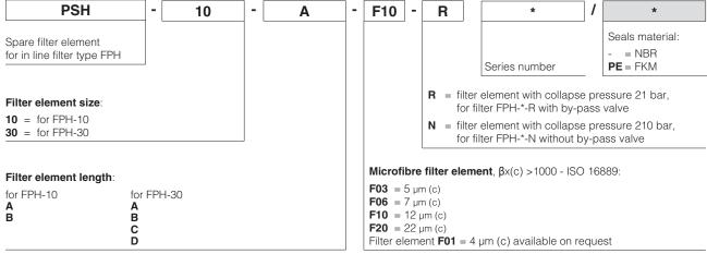
(1) Select the filter element according to the model code reported on the filter nameplate, see section 17
