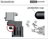
Mechanical pressure limiter setting - only AGMZO and AGRCZO with /P option For safety reasons the factory setting of the mechanical pressure limiter is fully unloaded (min pressure).
