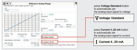
REMARK: Voltage Standard or Current 4..20 mA buttons do not act on Monitor output signal configuration! For Monitor output signal configuration browse to page Others - Monitor Outputs
