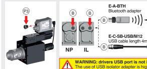
USB isolator adapter USB cable length 4m WARNING: drivers USB port is not isolated! The use of USB isolator adapter is highly recommended for PC protection (see GS500)
