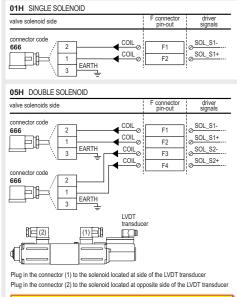
WARNING: for double solenoid valve pay atten- $\mathbf{\Lambda}$ tion to do not invert the connectors (1) and (2). If they are not inserted as shown in the example, the valve will not work properly and could cause eventual damages to the system.
