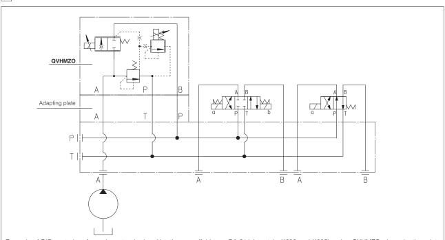
Example of P/Q control performed on standard multistations manifold type BA-214 (see tab. K290 and K295), using QVHMZO plus adapting plate (not supplied by Atos)
