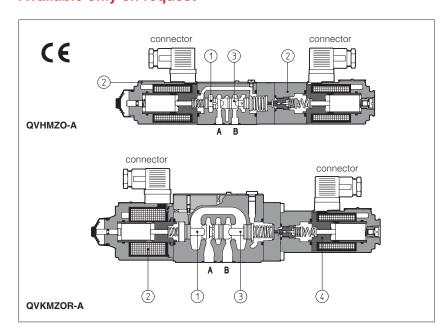
QVHMZO and QVKMZOR are proportional valves, direct operated, which provide indipendent pressure and 3-way compensated flow controls according to the electronic reference signals.
